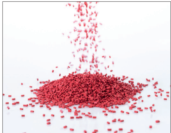
Fig. 2: Plastic granulate for injection molding or extrusion
